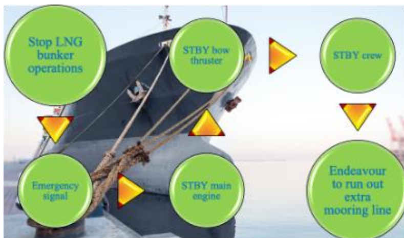
Fig. 4. Procedure in case of Mooring line failure
