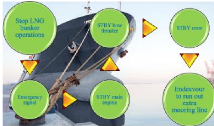
Fig. 4. Procedure in case of Mooring line failure
